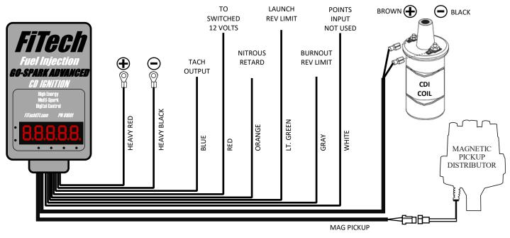
See Page 14 for Launch Rec Limit, Burnout Rev Limit, Nitrous Retard wiring details.
